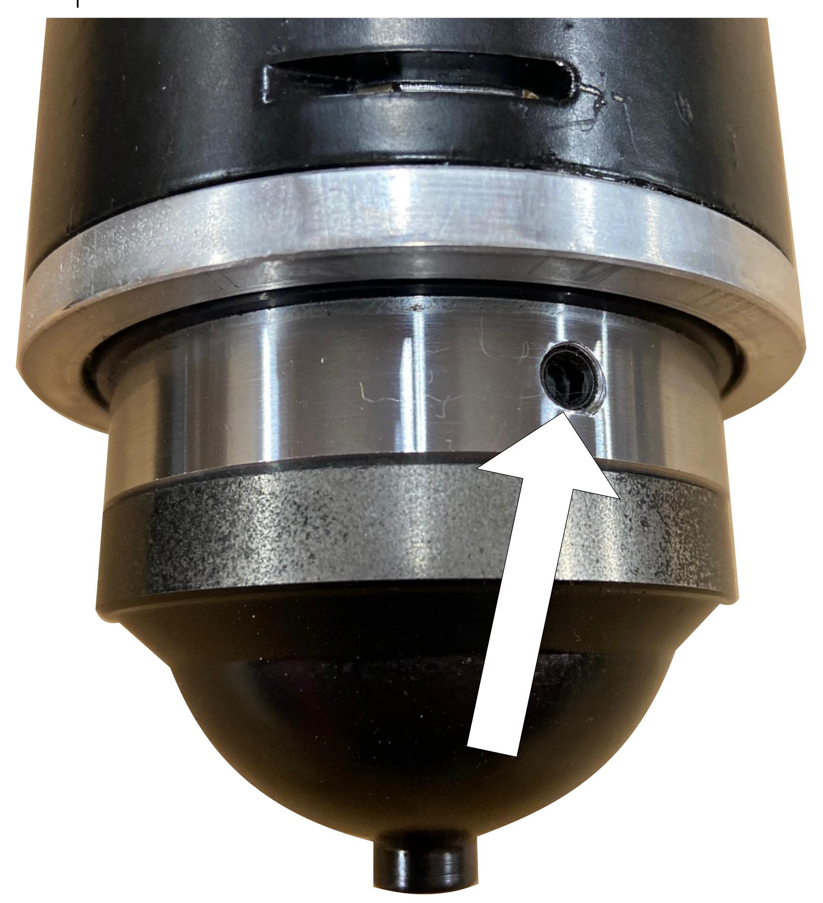
If you have a bolt on style pad, loosen the set screw shown, and remove the new base to reuse the original base.
