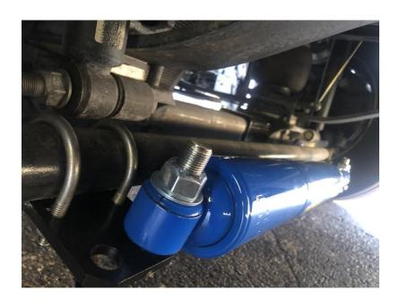
Step 5. Attach small end of SAFE-T-PLUS unit on 55-150B bracket using the bolt kit provided with the SAFE-T-PLUS unit (see picture).
