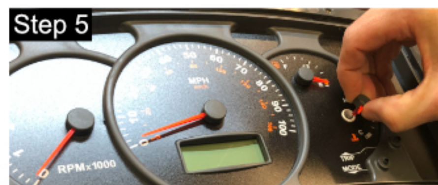
Remove the needles by rotating them completely around a few times to break them loose from the motor pins. Once they have been rotated, grab ahold of them as shown above and rotate them as you are pulling up on them firmly until they come off the motor pins. Set all of the needles aside for now.
