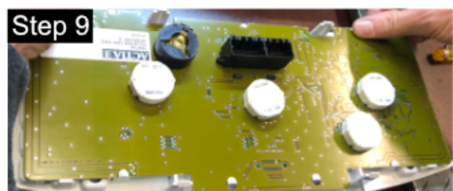
On the side of the board that has three white plastic tabs, gently lift on the board next to the plastic tab as you push out on the tab. Do this to each one of the tabs until that side of the board comes loose and lifts up.
