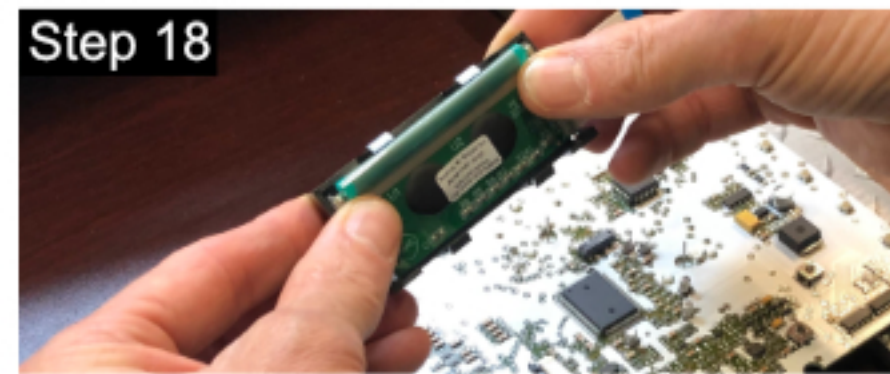
Snap the new screen into the bezel by aligning the white ribbon with the corresponding opening in the bezel. Place the side of the screen that does not have a ribbon around the edge into the bezel and with two fingers press the screen firmly into place. You will feel it snap into place.
