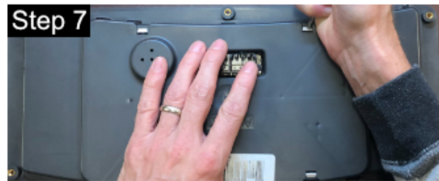
On the back of the case find the four white tabs. Locate the two that are closest to the plug and press toward the center of the case and down firmly until each of those two tabs release.
