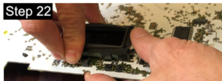
Lay the screen back over and install the bezel onto the board
