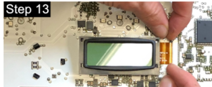
Using your finger nails, pull on the small tabs that are part of the dark grey retainer for the ribbon socket. Pull away from the white ribbon socket until the retainer comes to a stop.
