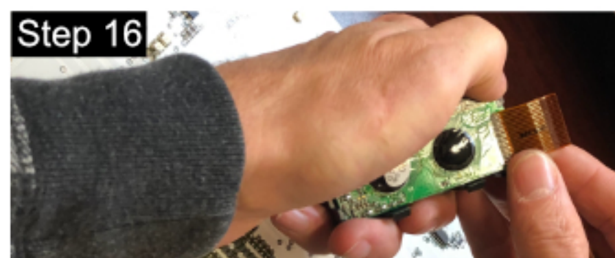
At the end of the bezel that has the ribbon coming out, holding the bezel as shown, press out on the bezel while pushing up on the screen to remove the screen from the bezel.
