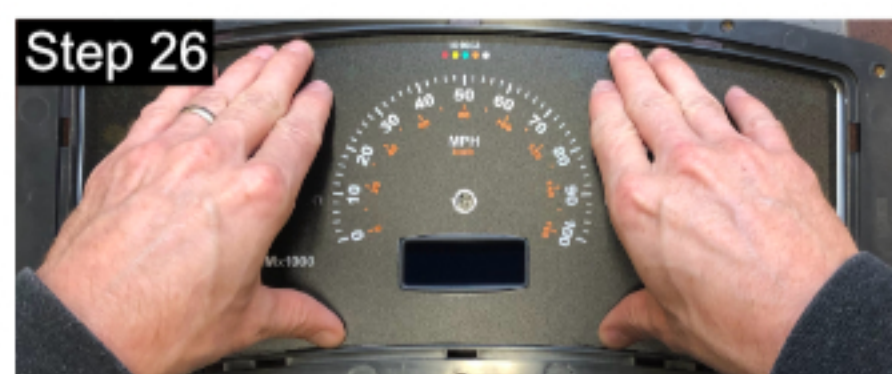
Be sure to press down firmly to snap the board assembly fully into the case. You will hear and feel it snap into place.
