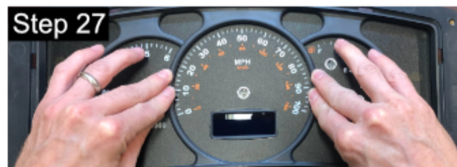
Once the board assembly is fully installed, you can reinstall the gauge surround plate. Make sure it also fully snaps into place.
