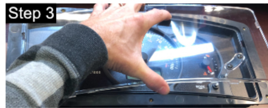
Once all of the tabs have been released, flip the cluster over and lift the lens out of the cluster case.
