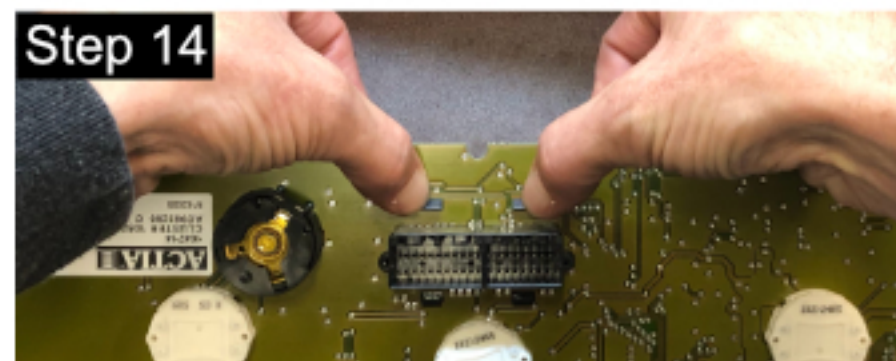
Turn the board over and press in and down on the tabs that hold the screen bezel to the board.
