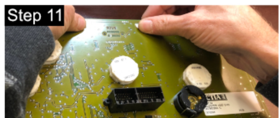
On the four remaining tabs on the other side of the board, you will want to do the same process as step 9. Press out on each of the four remaining white plastic tabs one at a time as you are gently lifting up on the board until the board comes loose.
