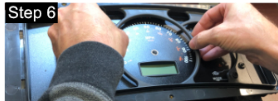
Remove the gauge surround plate from the face, by grabbing the surround as shown above in the photo and lifting straight up.
