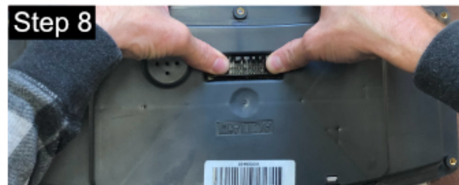
Press firmly down on the plug until the cluster board drops out of the case.
