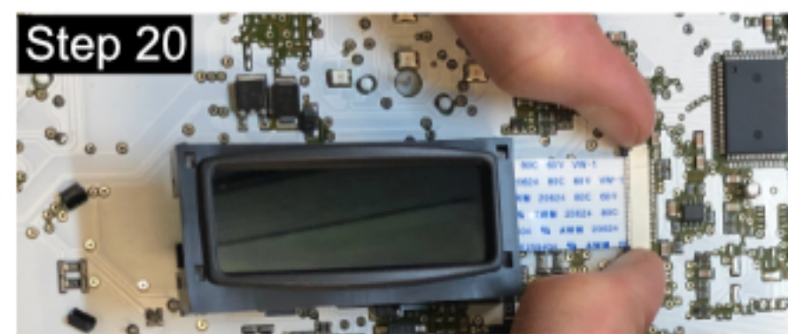
Lock the ribbon into the connector by using two fingers and pressing evenly toward the socket until the lock seats fully in place.
