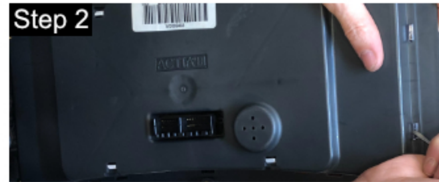
You will find the clear tabs all around the perimeter of the case.
