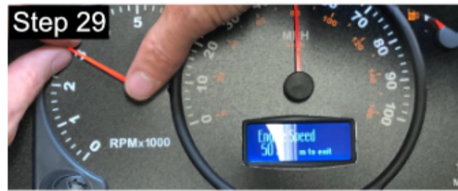
Using the steps listed below reinstall the needles as seen in the photo above. Start by GENTLY setting the needles on the motor pins so they are ready when you need to press them into place. All needles except the fuel gauge will be installed at the 50% point. The fuel gauge will be installed at the 100% point.
