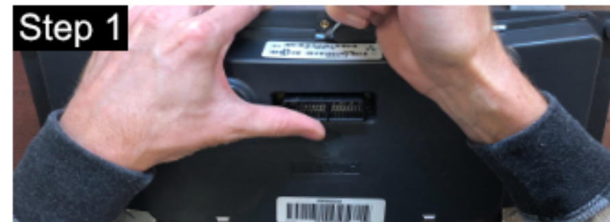
Once you have the instrument cluster removed from the vehicle, remove the lens cover from the cluster by pressing in and down on the clear tabs on the back of the cluster.
