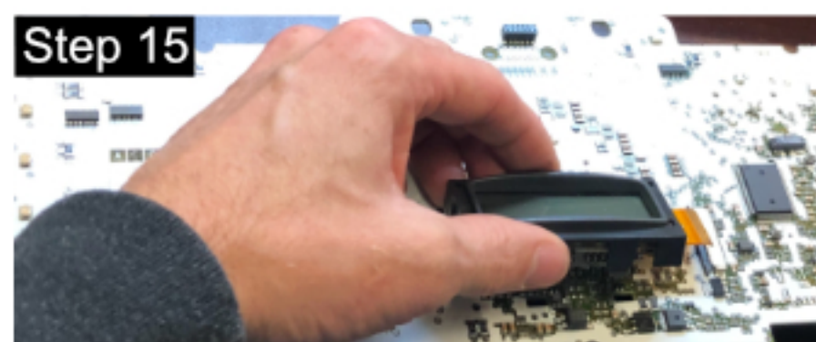
Once the bezel tabs are released, lift the bezel up and off the board.
