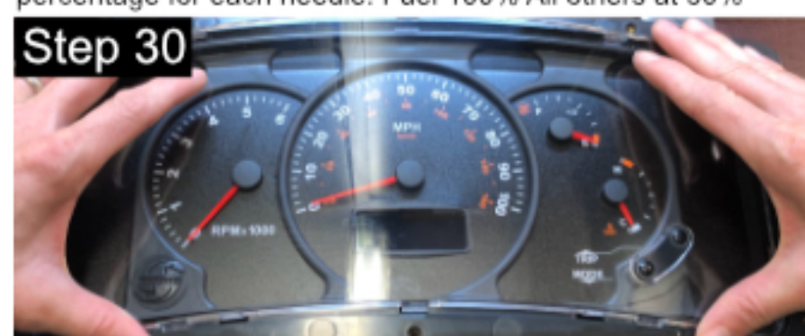
When all the needles are installed, make sure you unplug the cluster and then plug it back in and do the gauge test once more to verify they are correct. When done clean the lens and blow out any dust and reinstall the lens. All done!
