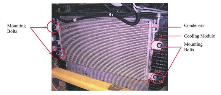
10. Loosen and Remove the 4 off Bolts that attach the Condenser to the Cooling Module.
