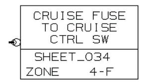
The top portion of the box gives you the details of the circuit. Below the line, the point where the circuit continues is shown along with the grid locator. Use the grid locator in the same way that a road map is used to pinpoint the location.
